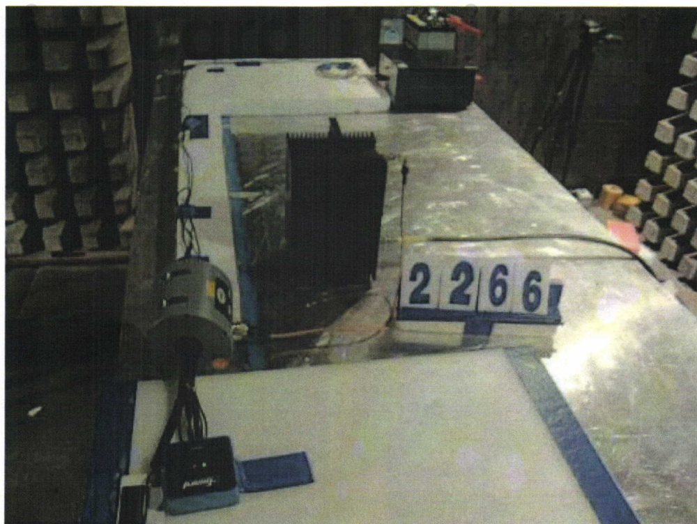
FIGURE 7 - The test setup picture for BCI.
