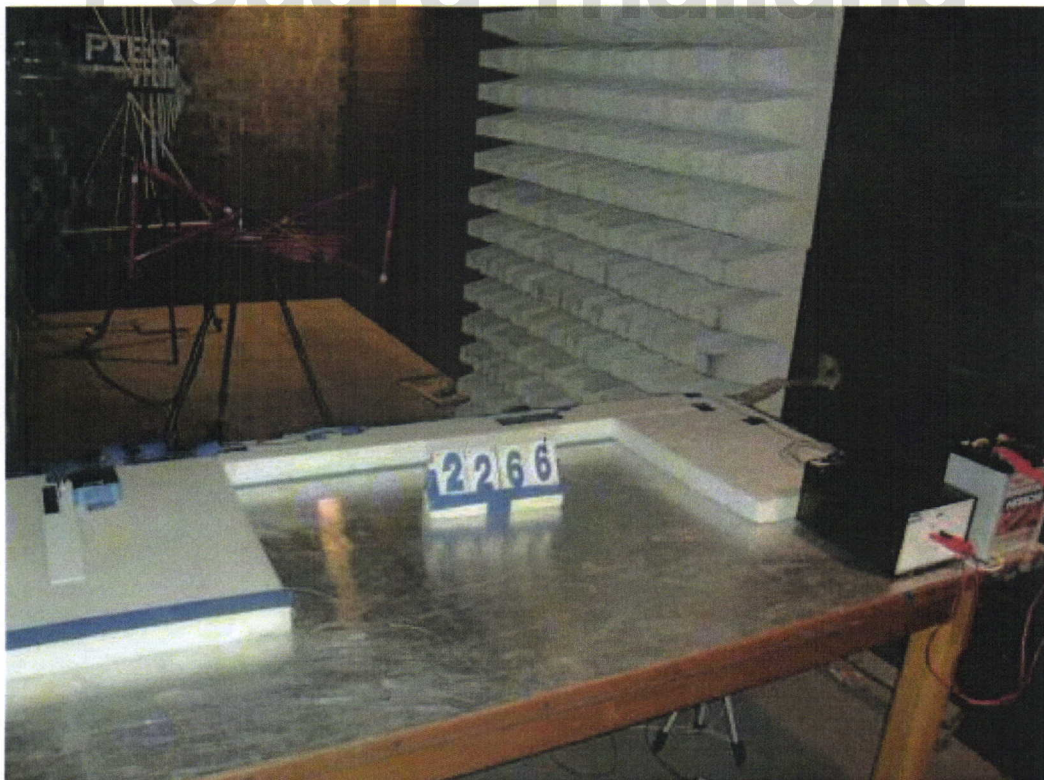
FIGURE 3 - The test setup picture for Radiated Emission.
